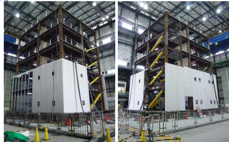
Full-Scale 5-story Steel building with Steel Damper
